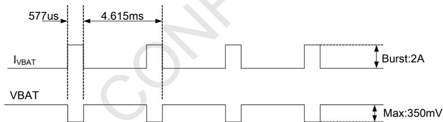
**Figure 9: VBAT voltage drop during transmit burst**
