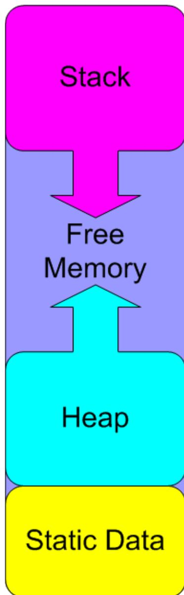
Most memory problems occur when the stack and the heap collide. When this happens, one or both of these memory areas will be corrupted with unpredictable results. In some cases it will cause an immediate crash. In others, the effects of the corruption may not be noticed until much later.
