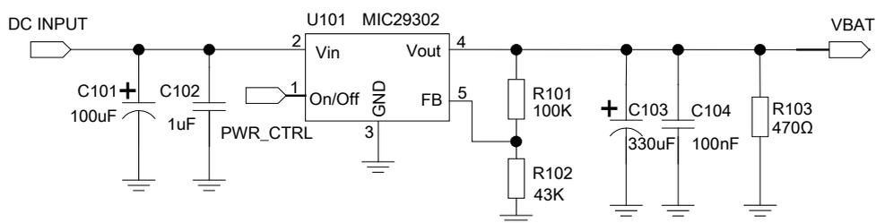
Figure 7: Reference circuit of the LDO power supply
