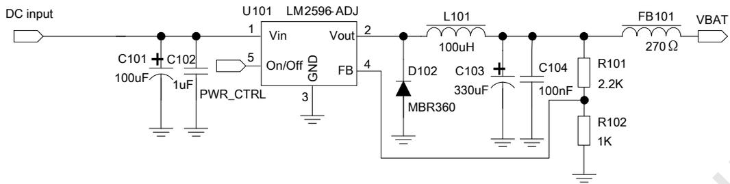
**Figure 8: Reference circuit of the DC-DC power supply**
