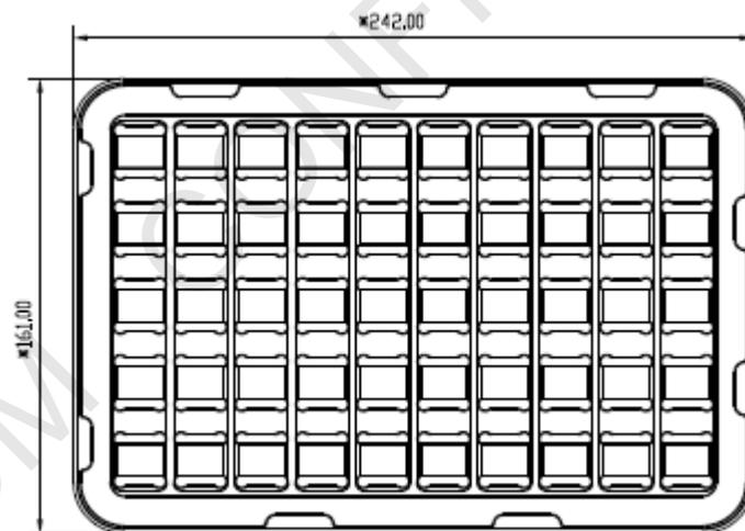
Figure 44: Module tray drawing
