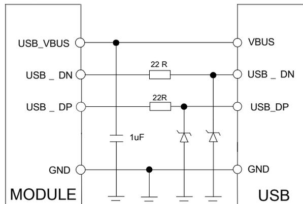
**Figure 24: USB reference circuit**
