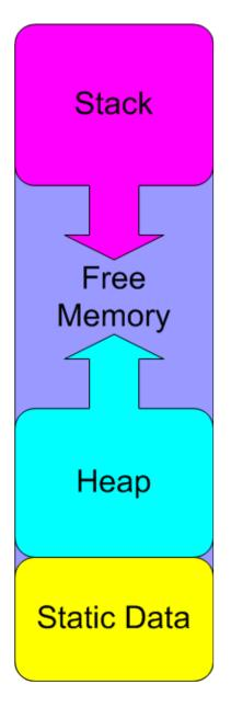
Most memory problems occur when the stack and the heap collide. When this happens, one or both of these memory areas will be corrupted with unpredictable results. In some cases it will cause an immediate crash. In others, the effects of the corruption may not be noticed until much later.
